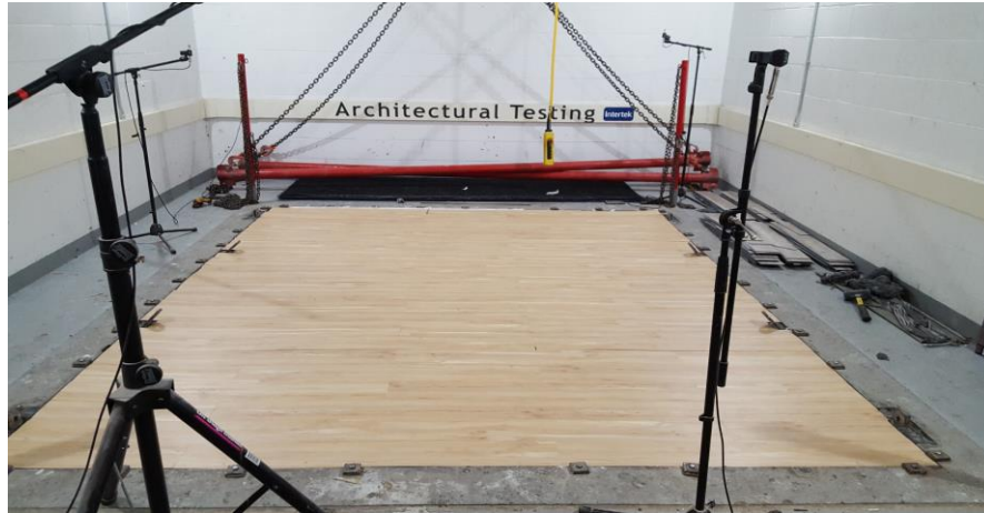
Source Room View of Test Specimen Installation
